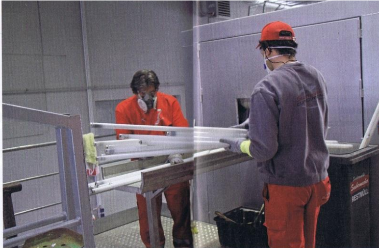
The mercury and rare earth metals-containing layer of powder inside the fluorescent lamps is sucked out via a series of filters in the plant and collected in closed drums.
